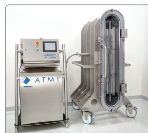
Figure 6: ATMI LifeSciences Helium Integrity-Testing platform
